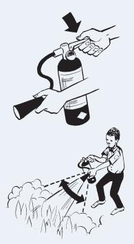
Squeeze the handle to discharge the extinguisher (stand approximately 2.5 m [8 ft] away).
