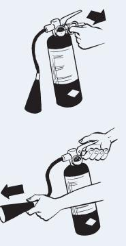
**P**ull the pin at the top of the extinguisher.
