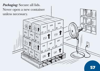
*Circulation:* Use a fan to circulate fresh (outside) air. In bigger storerooms you may need a ceiling fan. Standing fans are more useful in smaller storerooms. This requires electricity and some maintenance.
